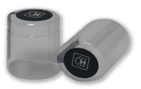
The shrinkable protective hood is made of PVC plastic and can replace all other protective hoods, plugs, caps and plugs. The protective hood is threaded onto the mounted clutch and then heated quickly with a heat gun, the plastic shrinks around the clutch and protects the hose and clutch from dirt. The protective cap is quickly removed using a perforated strip.
